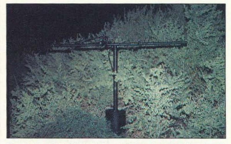
Photo B. Kevin Kelly N6QAB built this motorized quad when he put on a long-distance hunt in the Albuquerque area. It automatically turned back and forth to vary the signal reflections from the nearby hills.
